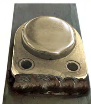
Correctly welded across the end of the tab
